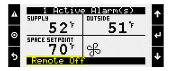
"Remote Off" means that the Remote Start input on the unit's controller is not satisfied. On most units, the Remote Start input is associated with the field-wired contact labeled, "S1".
