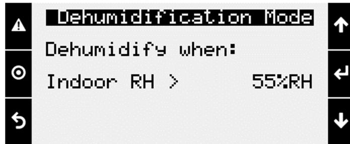
5. Use the Down arrow key to navigate to the Dehumidification Mode Unoccupied Mode screen. This screen will indicate when the unit will enter a dehumidification mode when the unit is in an unoccupied mode. The specific setpoint/s (Example: 60%RH & 55°F) at which the unit will enter dehumidification mode can also be edited on this page.
