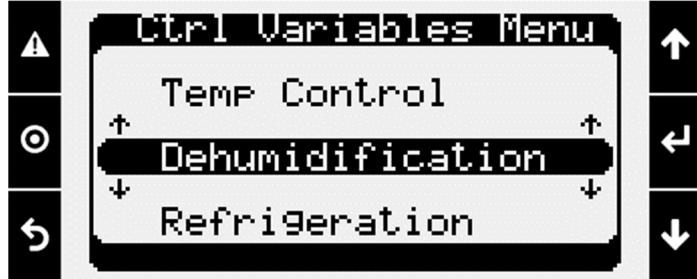
4. Use the Up/Down arrow keys to navigate to the Dehumidification Mode Screen. This screen will indicate when the unit will enter a dehumidification mode when the unit is in an occupied mode. The specific setpoint/s (Example: 55%RH) at which the unit will enter dehumidification mode can also be edited on this page.
