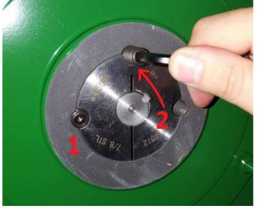
3. Tighten set screw #2 (see below) until the wheel disengages from the bushing. The disengagement occurs when the wheel separates from the bushing approximately 1/8".
