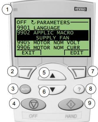
8. Continue accessing and editing all the parameters that you need to. For a complete list of drive parameters and their meanings, please reference the ABB ACS320 user manual. For inquiries relating to unit-specific parameters such as the speed references, please reach out to DOAS Technical Support.
