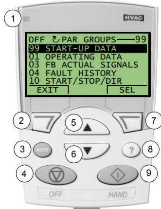
5. Use the up/down buttons (5 & 6) to scroll through the parameters. Highlight the desired parameter and use the soft key (7) "EDIT" it.
