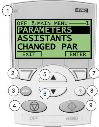
4. Use the up/down buttons (5 & 6) to scroll through the parameter groups. Highlight the desired parameter group and use the soft key (7) to select it.
