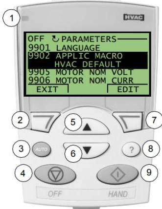
6. Use the up/down buttons (5 & 6) to change the parameter value and use the soft key (7) to "SAVE" it. Alternatively, use the soft key (2) to "Cancel" and exit back to the parameter list.
