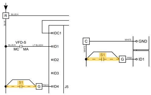
4. Remove the factory jumper connection between the specified terminal blocks (**R to G** or **C to G** depending on your unit's wiring diagram). This jumper may be a wire connecting the two terminal blocks or an orange jumper bar that fits into the front face of the terminal blocks like below.
