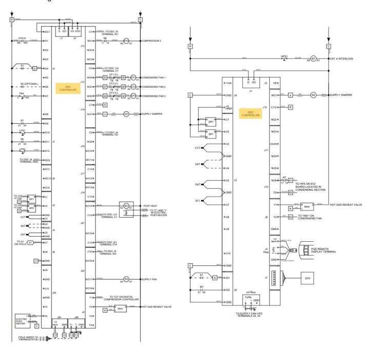
3. Find the normally open contact S1 on the low voltage electrical schematic. It should show the contact as being field wired, with a factory jumper wire bypassing it. Examples of the S1 contact on low voltage electrical schematics are shown below.
