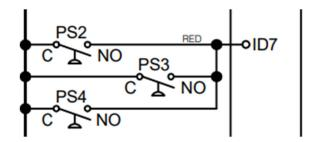
The filter pressure switches are wired in parallel with each other so that any one switch closing will trigger a dirty filter alarm. The unit controller is looking for this switch closure on its input. In this example, the controller is looking for switch closure on digital input ID7. The unit's supply fan should be running while troubleshooting.
